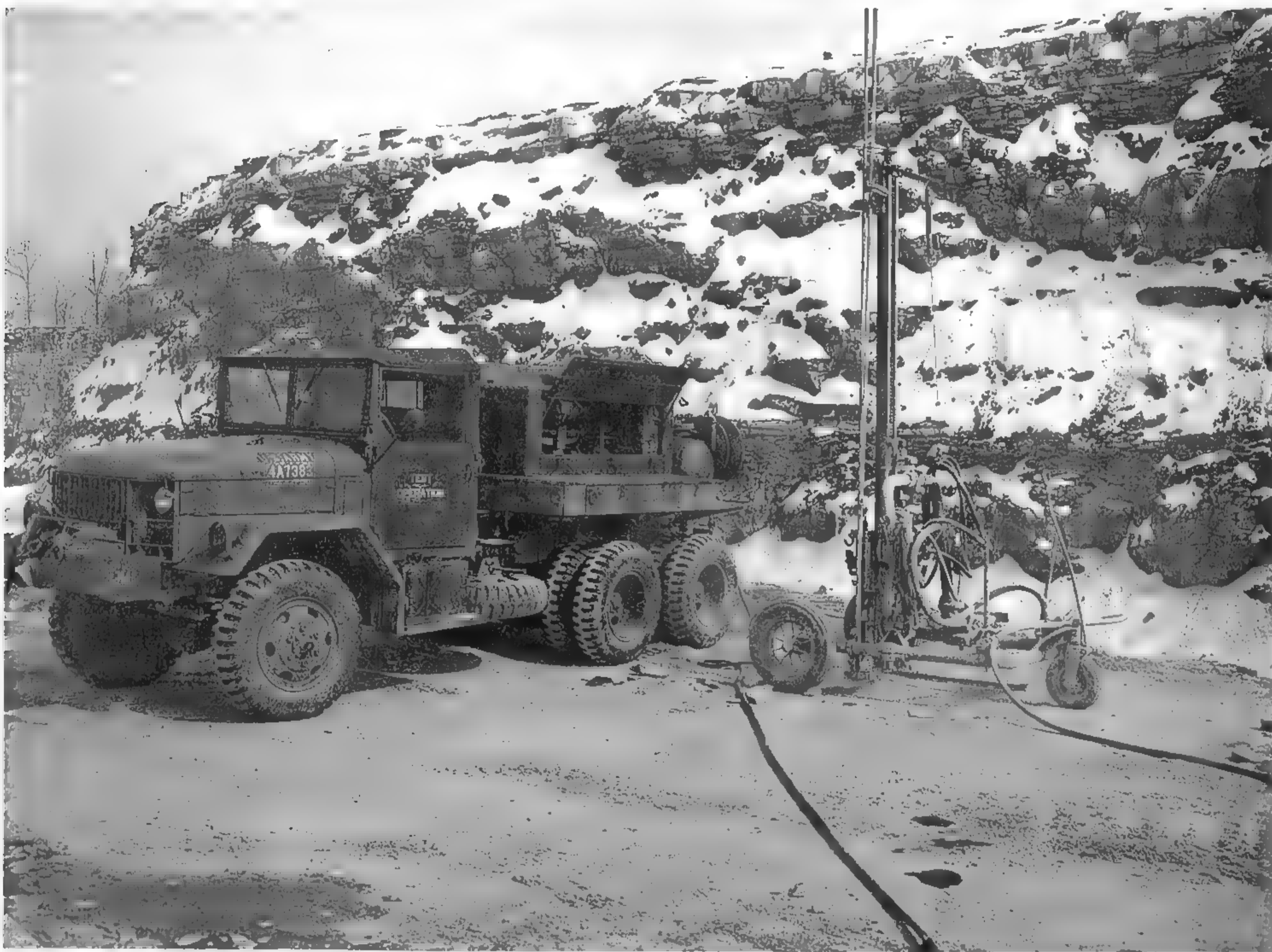
The 210 WDS, like the 210G1, carried an extensive assortment of tools, but these units could also be used to supply air to other equipment. (Photo courtesy of United States Army Engineer School History Office)
